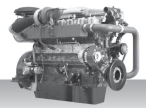
6-cylinder, 4-stroke, water-cooled diesel engine, with direct-injection, turbocharger and air-cooler.
